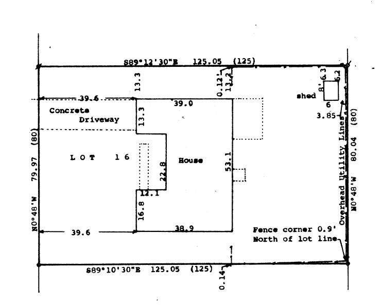
Scale - 1" = 20' o = 1" Iron Pipe Found #= 14" Iron Pipe Found Bearings referenced to the recorded bearing of N0°48'W along the east line of Tyrell Avenue Survey ordered by: Assured Realty, Inc 50 West Geneva Williams Bay, WI 53191 (0.00) = recorded distance
